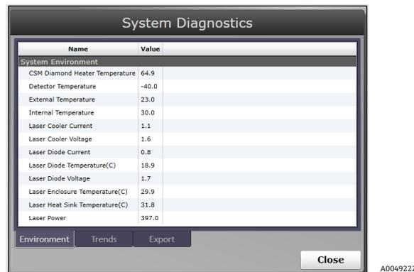
Figure 86. System diagnostics environment tab
