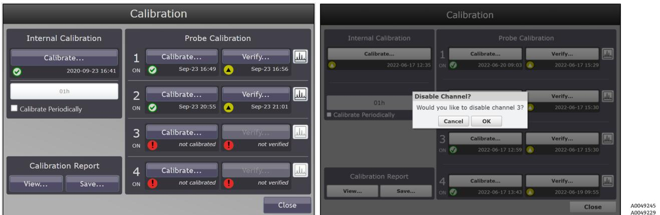
Figure 83. Channels 3 and 4 show unused/uncalibrated and the disable channel 3 prompt
