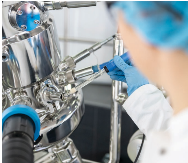
Memosens CPS61E for process control in fermentation processes and control of culture growth
