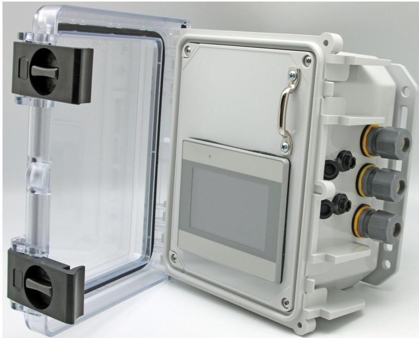
Clear Hinged Latched Protective Door provides outstanding NEMA 4X protection for touchscreen HMI from environment. In order to access the internal components of controller simply remove the two far right screws and open with the pull handle.
