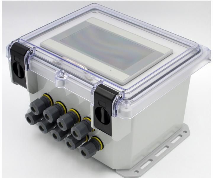
Clear hinged latched door provides outstanding protection for advanced touchscreen HMI from environment as part of NEMA 4X rated assembly. To access internal components of controller simply remove two top screws & open with pull handle. One left are 6 each NEMA 6P rated female snap panel mount connectors for plug & play smart digital sensors and 5 each cable glands while on right are 9 each cable glands (all factory installed).
