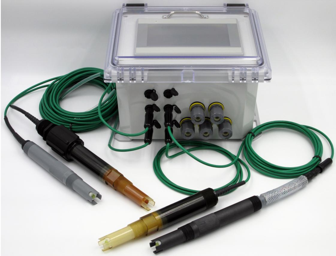
Six (6) channel HiQDT-CTRL-6CH controller shown with 4 each smart RS485 MODBUS RTU pH sensors connected (two top ports are unused). Controller is NEMA 4X when the door is latched. Hot swappable sensors with plug & play snap connectors are NEMA 6P rated when interfaced. The 3 & 6 channel controllers with 7.0" touchscreen are available in configurations that are suitable for hazardous Class I, Division II locations.
